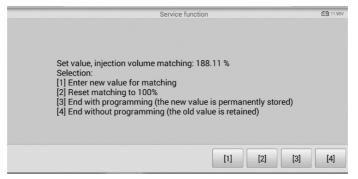
Figure 5-24 Sample Injection Rate Screen
