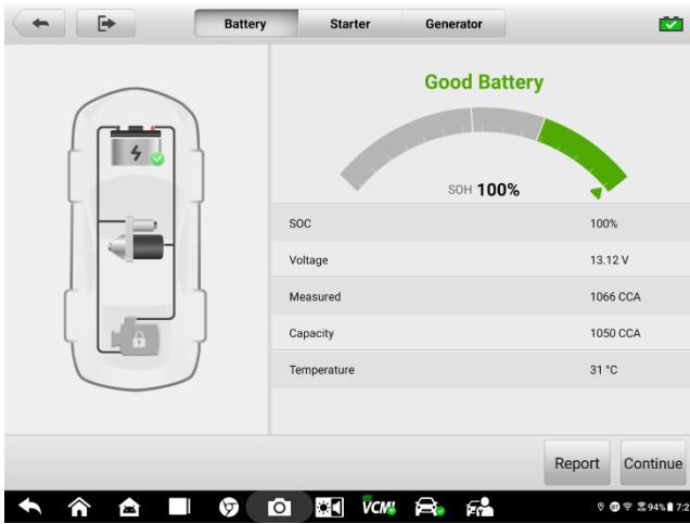
Figure 10-7 Battery Test Results Screen
