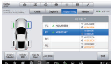
Program Success (MX-sensor ID is copied from the sensor ID saved in ECU)
